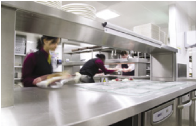
Left: Ross's kitchen was designed so that the hot and cold passes are close together, ensuring he can see all the plates going out
